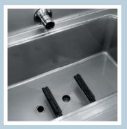
A one piece deep drawn pressed tank with fully rounded corners, sloped towards the drain to prevent dirt build up, provides fast drainage in only a few minutes. Pressed tanks, with no welded points offer a guaranteed water tight solution.
