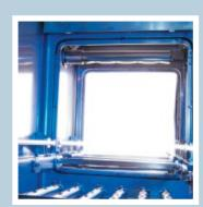
The washing chamber is without internal pipes and therefore no hidden dirt traps.
