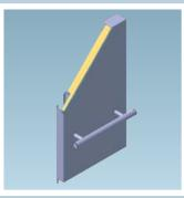
The double skinned counter-balanced doors with 35mm thick injected foam insulation adds strength as well as reduces noise and heat loss.
