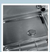
Pre-wash & wash tank filters feature holes smaller than the concave anti-block wash nozzles so that large food particles will not enter and block the wash system.
